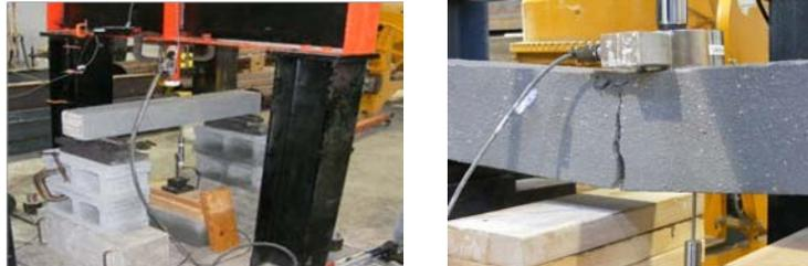
**(a)** **(b) FIG. 4. (a) Flexural fatigue test system, (b) Piston applying force to load cell**
