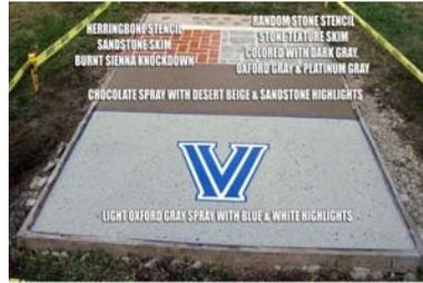
**FIG. 8 DCO on outdoor field slab**
